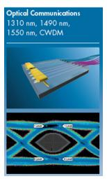
The latest generation of communication systems and modules require components with extremely low power dissipation, small form factors and high performance. VERTILAS offers innovative laser solutions for 1310 nm, 1490 nm, 1550 nm, CWDM and DWDM. VERTILAS' TOSA (Transmit Optical Sub Assembly) packaging with LC receptacle features an integrated monitoring diode and a typical power dissipation of less than 30 mW.
